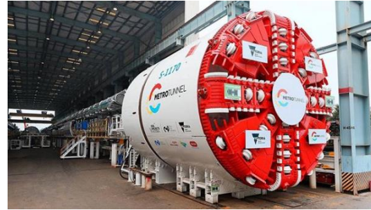
Tunnel Boring Machine
