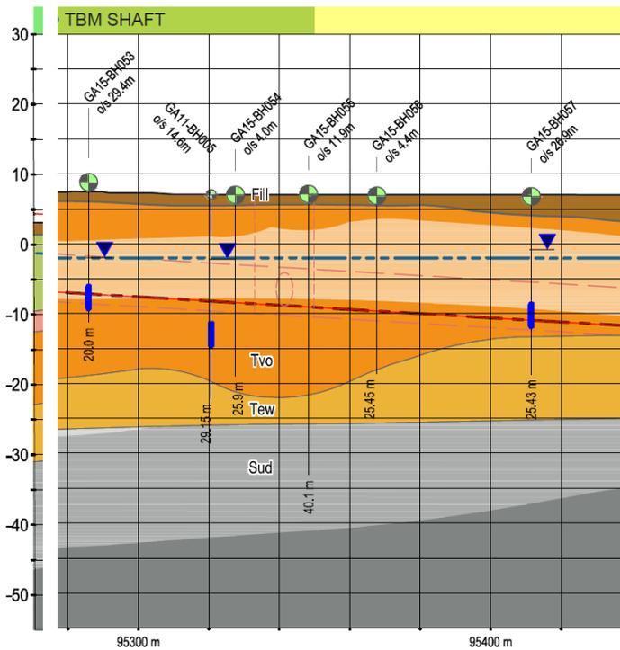
Figure 1 Extracts from Geological Long Section Drg 1525532-331-R-003 with plan showing current approximate surface levels
