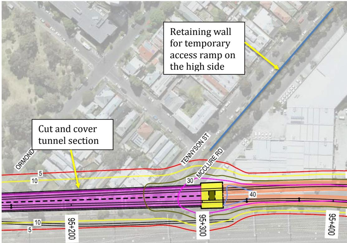
Figure 2 Extract from Ground Movement and Land Stability report, MMR-AJM-UGAA-DR-NN-500431, Settlement Contours, Sheet 2 of 15, marked up to show the line of the retaining high-side wall of the retaining wall option for the ramp
