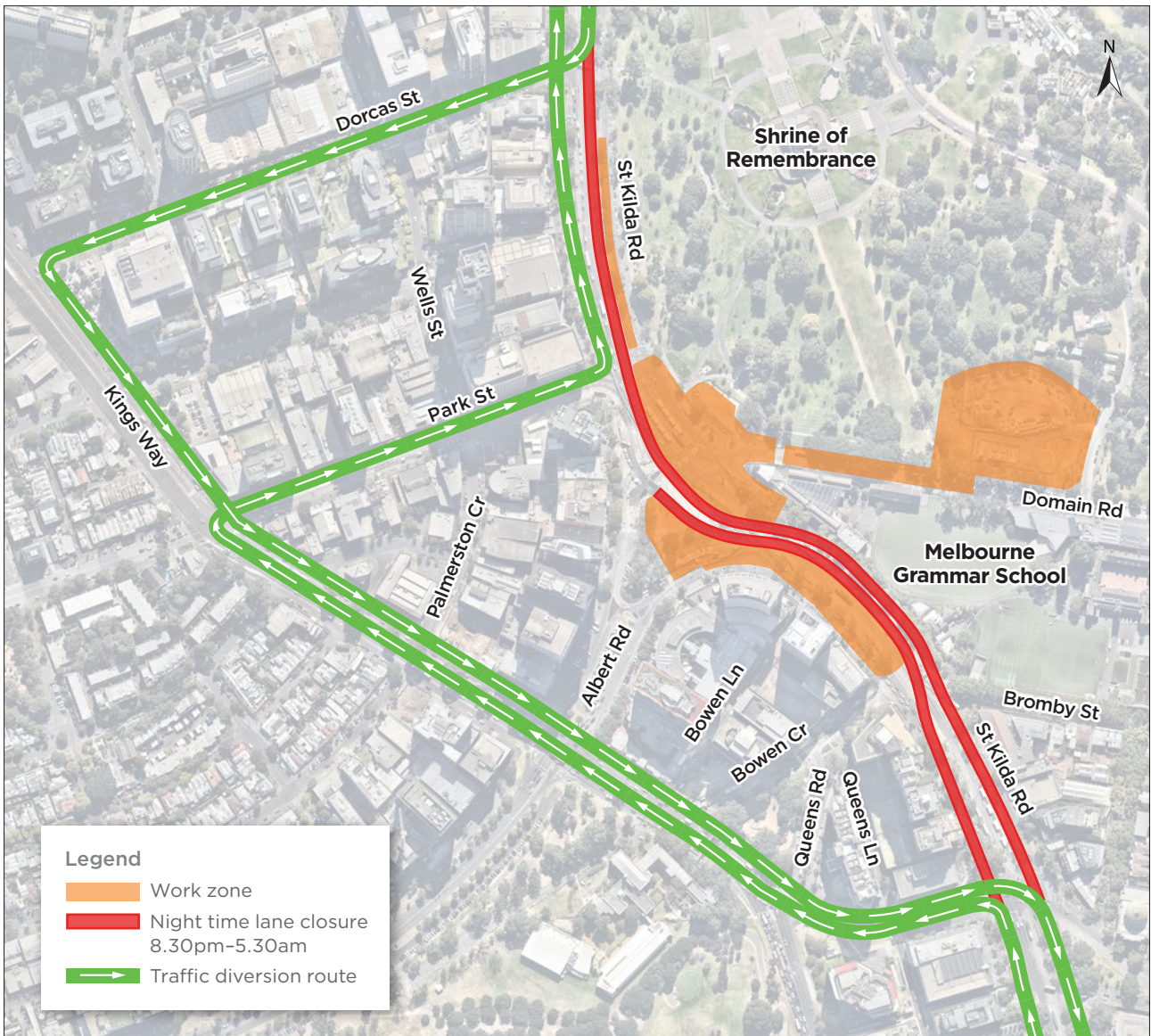
Overnight St Kilda road closures and traffic diversion, indicative only.
