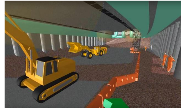
Tunnel excavation works under the roof slab
