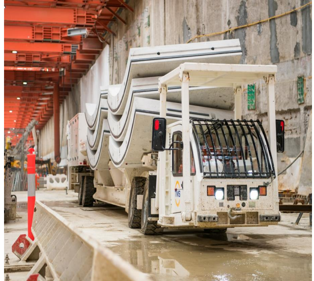
Multi-service vehicle (MSV) carrying lining segments
