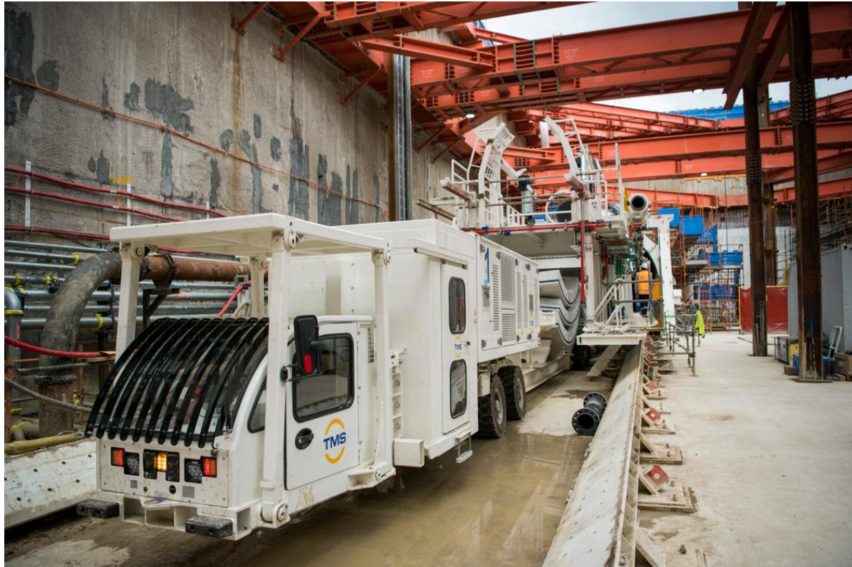
Multi-service vehicle (MSV) carrying lining segments
