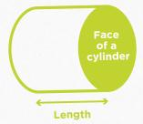
Pi  $(\pi)$  is used to calculate the area of the face. Pi is the ratio of a circle's circumference to its diameter. Regardless of the size of the circle, Pi is always the same number, approximately 3.14.
