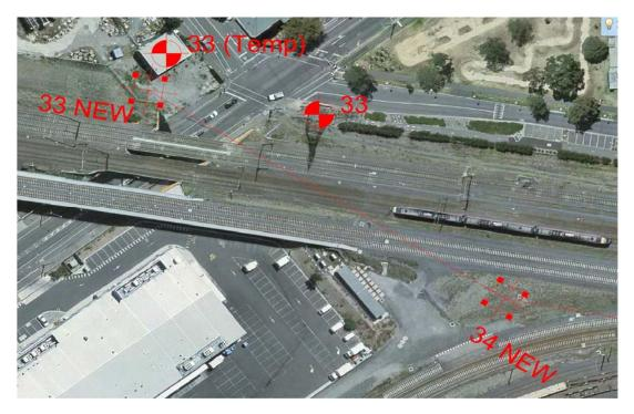
Figure 3: Indicative temporary transmission tower locations for Tower 33 and new Tower 34
