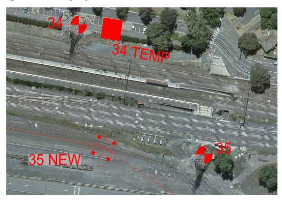
Figure 4: Indicative temporary transmission tower locations for Tower 34
