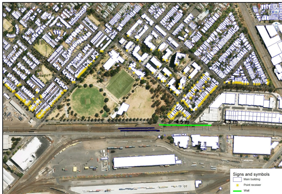
Figure 13-4 Example operational noise mitigation for Concept Design
