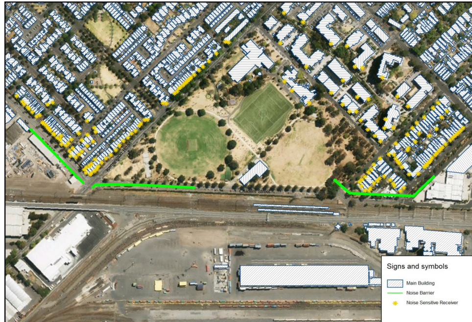
Figure 13-3 Proposed construction noise mitigation
