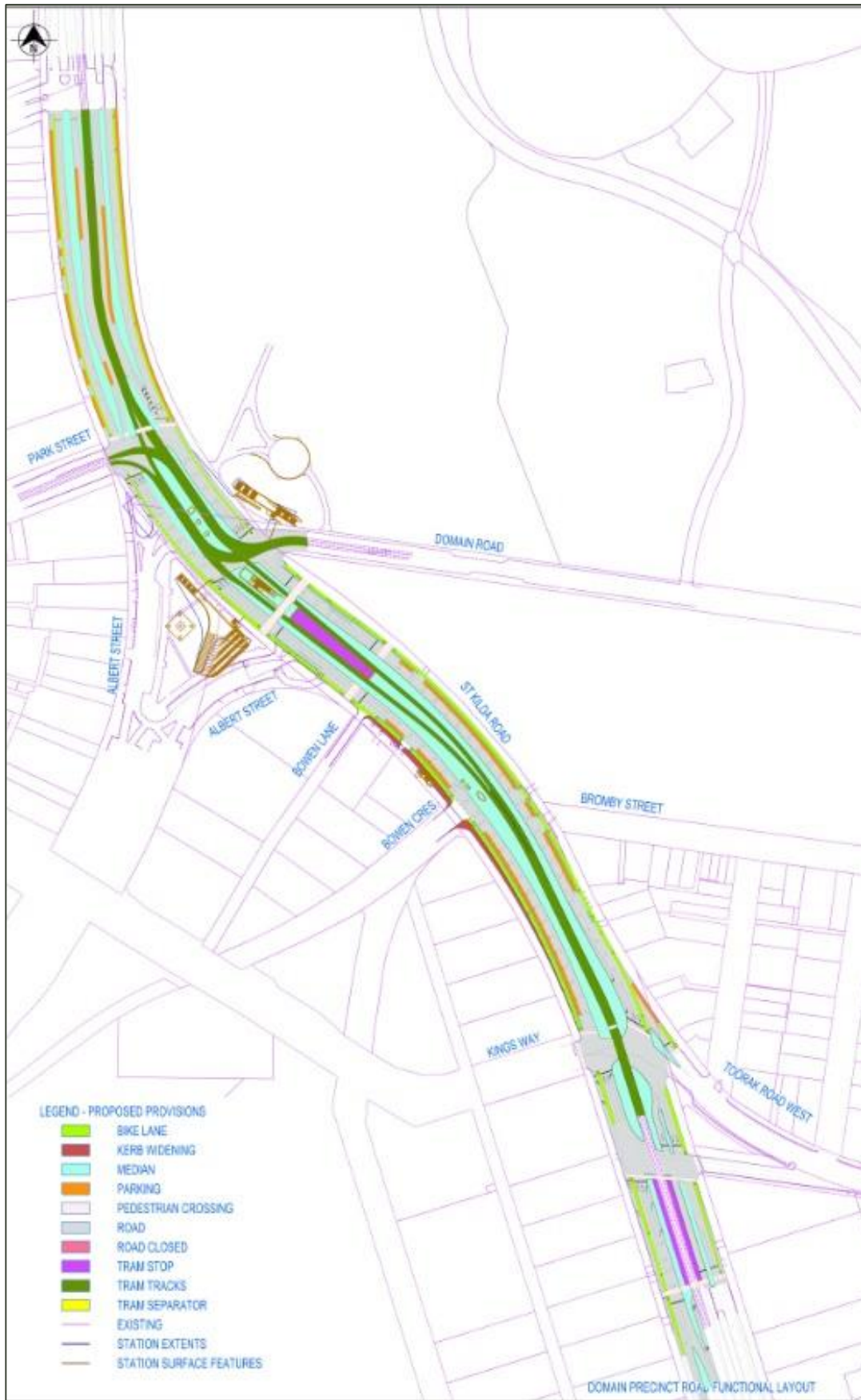
Figure 3-14 Road functional layout around Domain station
