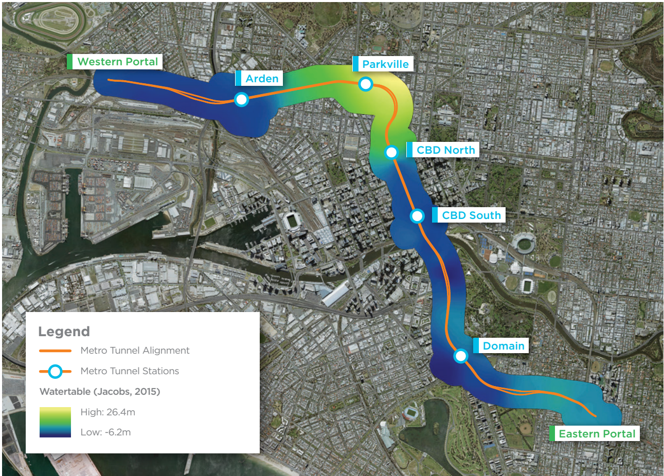
Figure 10: Map identifying depth of water table over the Metro Tunnel project area. Areas with the shallowest water table (within 6m of the surface) are shown in dark blue (Melbourne Metro Rail Project Environment Effect Statement, May 2016 Technical Appendix O)
