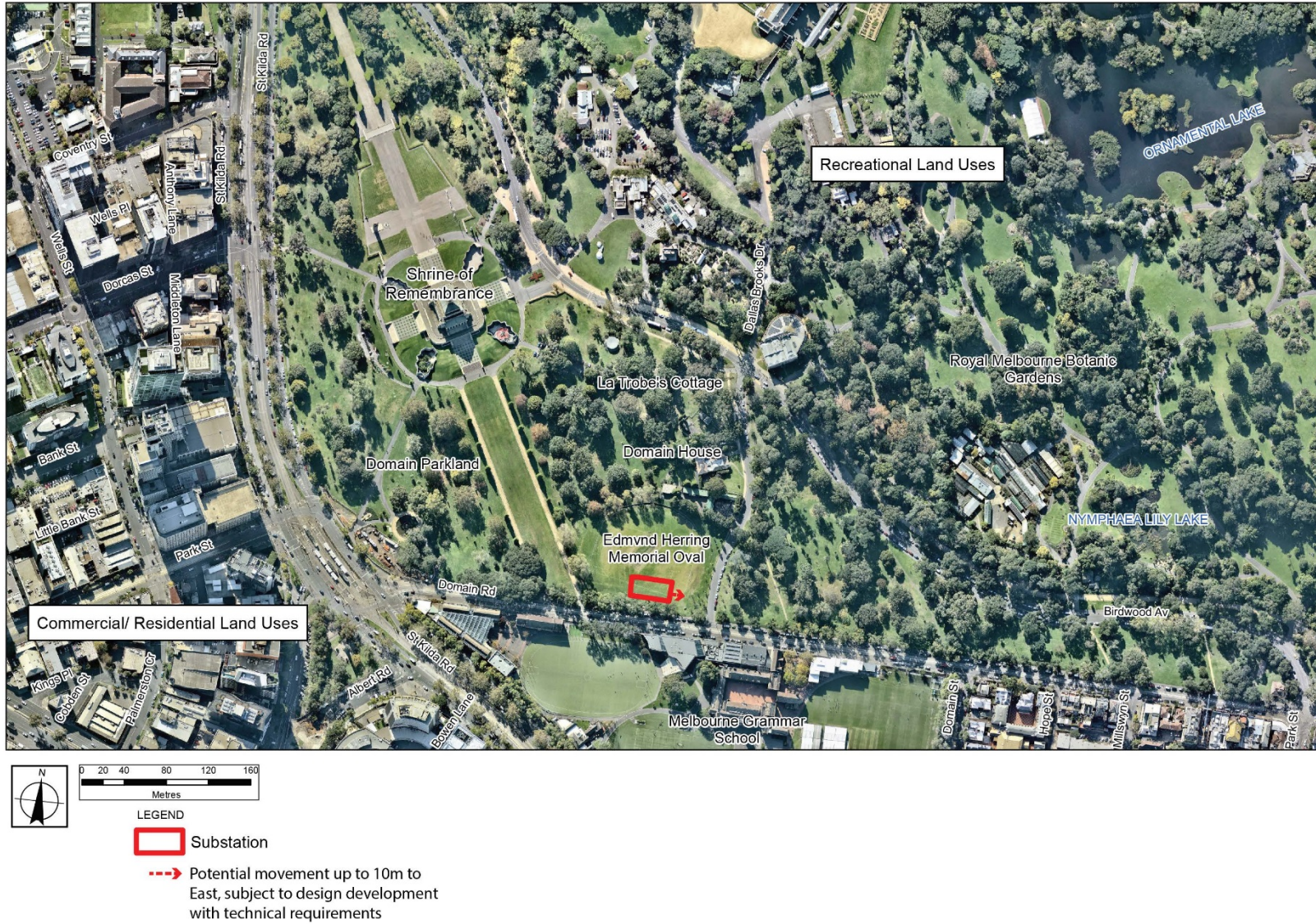
Figure 3 Domain temporary substation location and site context
