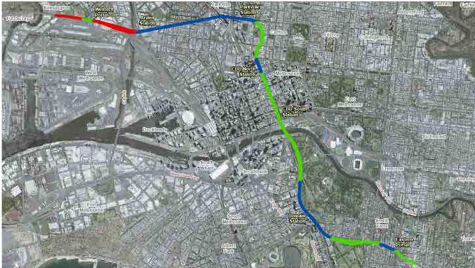
Figure E.49: Graphical representation of the extent of trackform mitigations (red - 'standard attenuation', green - 'high attenuation', blue - 'very high attenuation')
