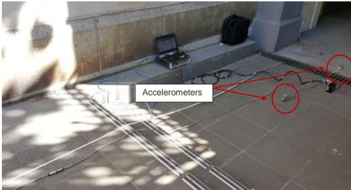
Figure E.7: Surface vibration measurement above the City Circle Loop Ch 5039 (State Library)
