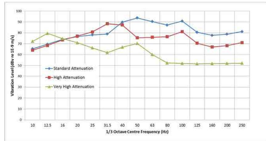
Figure E.5: Tunnel wall vibration source spectra for standard attenuation, high attenuation and very high attenuation track forms (95<sup>th</sup> percentile train passby  $L_{Vmax,slow}$  referenced to a train speed of 80kph)
