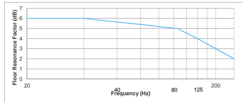
Figure E.9: Floor resonance amplification factors
