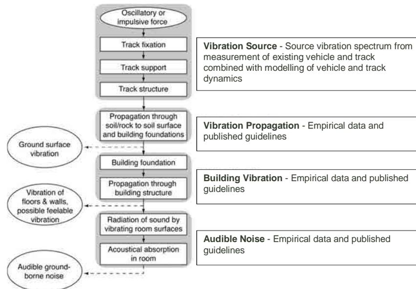
Figure E.3: Operational vibration and ground-borne noise modelling process (source - FTA guideline)
