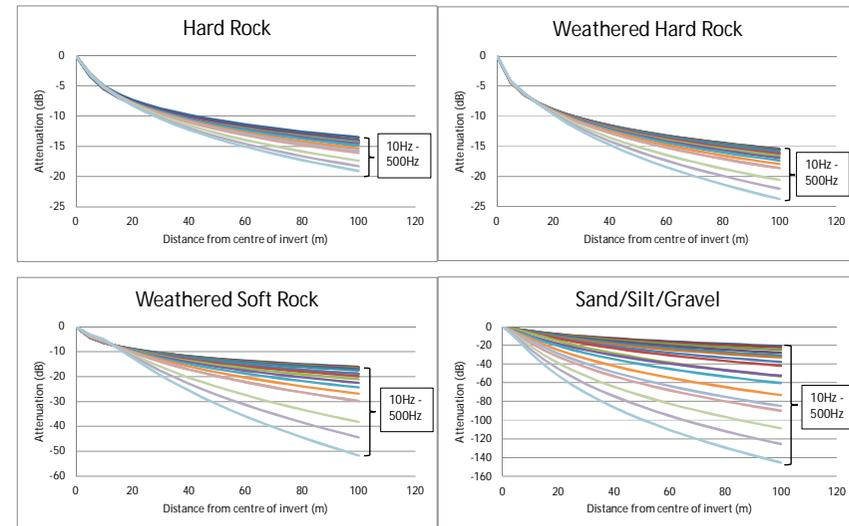
**Figure E.6: Ground vibration attenuation versus distance from centre of invert for rail vehicles operating in a tunnel**
