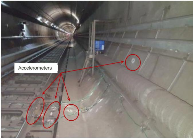
Figure E.4: Vibration transducer installation at a single tunnel cross-section (Ch5039)
