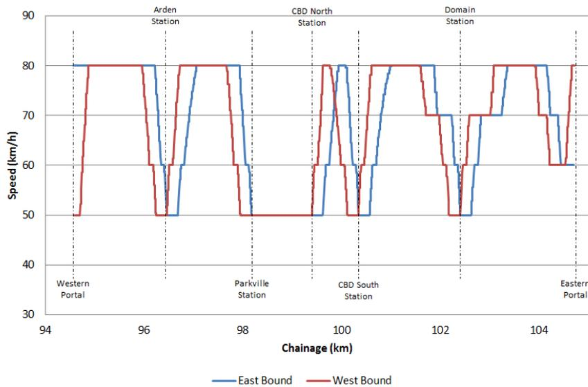
Figure E.2 – Speed profile (with 50km/h speed floor through stations)
