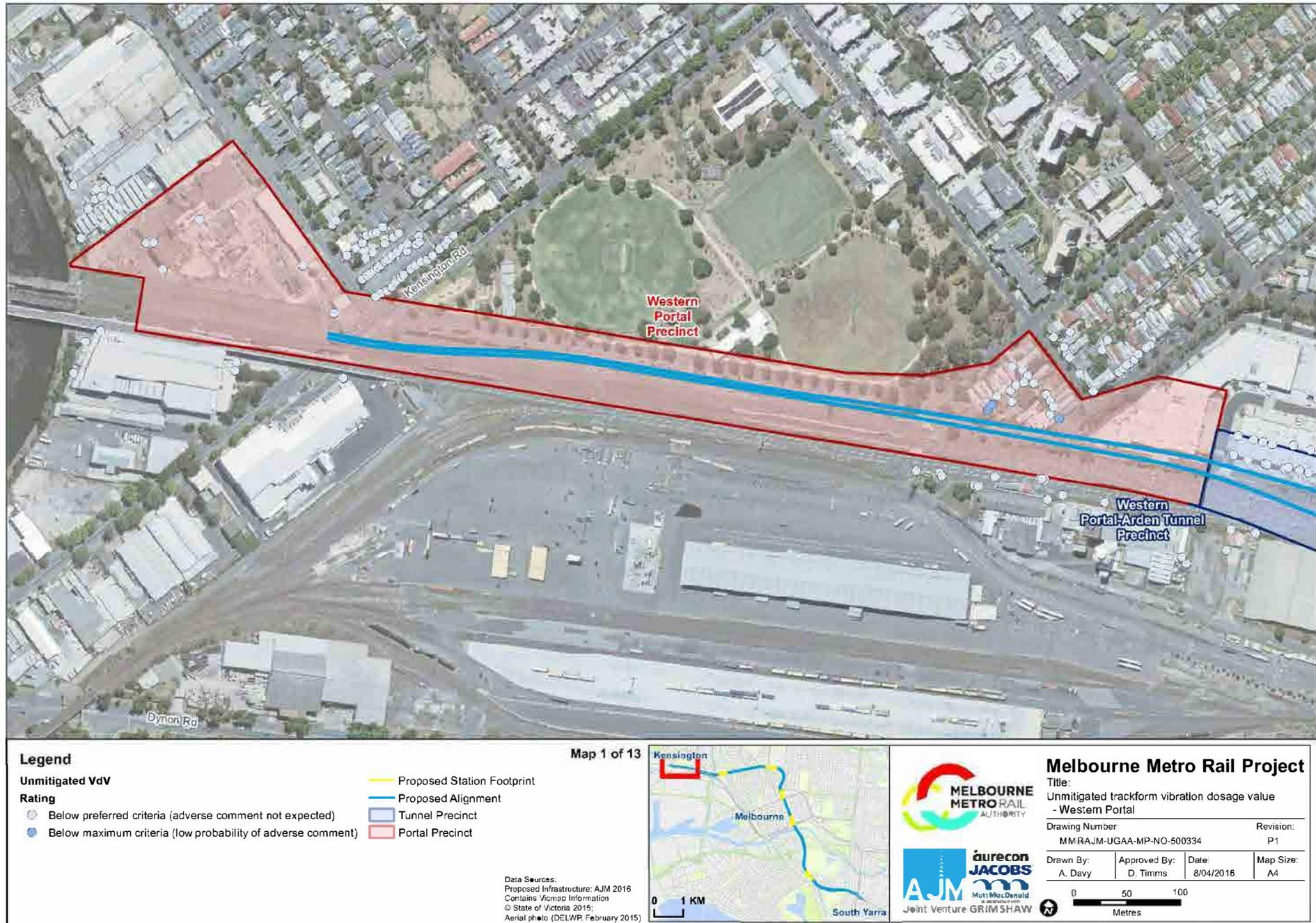
Figure E.10: Unmitigated Vibration Levels (VDV) for Human Comfort due to Trains in Precinct 2: Western Portal
