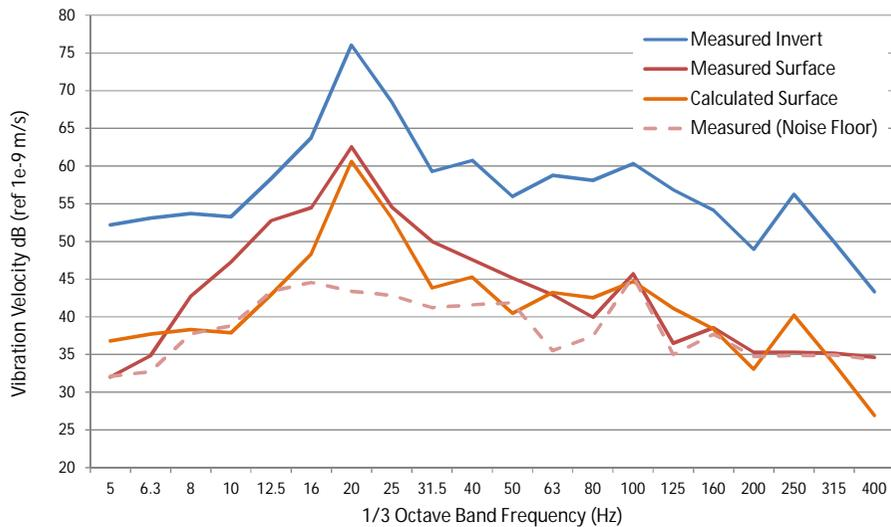
Figure E.8: Average vibration spectrum at the tunnel invert and surface at Ch 5039 (State Library), reference speed 50 km/h
